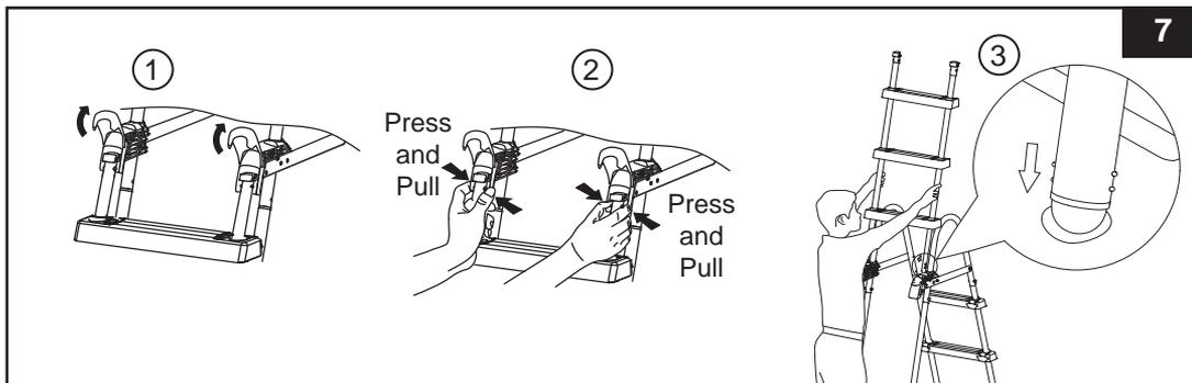
**9. Removing the steps from the secured position** (refer to figure 8):
