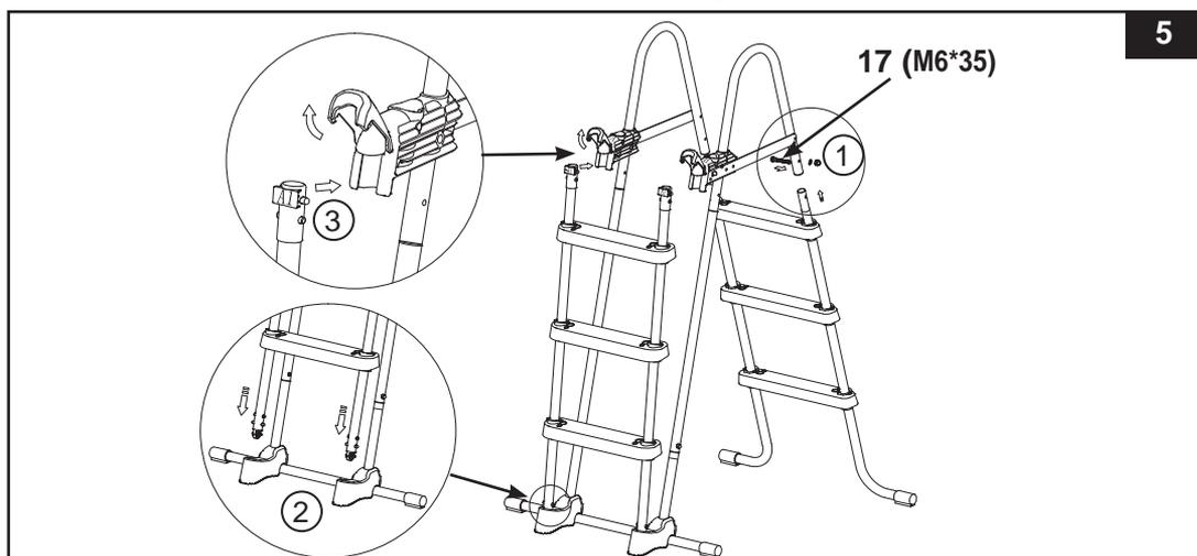
**IMPORTANT:** Do not fully tighten fasteners until last assembly operation.
